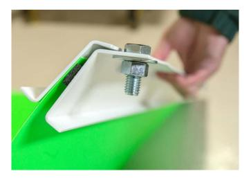
Using two people (one at each hex cap screw) carefully lift the green-screen assembly up to the angled mounting brackets and drop the two bolts through the holes in the mounting brackets. Make sure that you do not fold or crease the Virtual Green® Pro Matte® material during this step.
